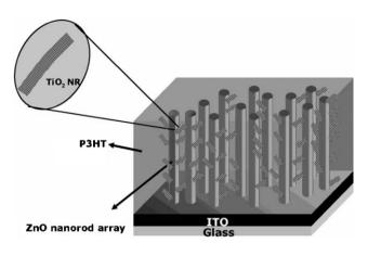
Fig. 1 Schematic representation of the 3D nanostructured photovoltaic device based on the ZnO/P3HT:TiO<sub>2</sub> hybrid material.
