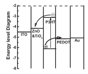
Fig. 4 The corresponding energy levels of the nanostructured photovoltaic device based on  $ZnO/P3HT:TiO_2$  nanorod hybrid.
