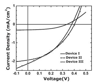
Fig. 7 Photovoltaic performances of devices with different configurations. Device I: (ZnO/P3HT); Device II:  $(ZnO/P3HT:TiO_2)$ ; Device III:  $(ZnO/TiO_2 nanorods/P3HT:TiO_2)$ .
