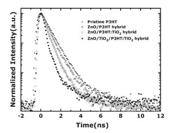
**Fig. 6** Time-resolved photoluminescence spectroscopy for the samples consisting of pristine P3HT (Sample A), ZnO nanorods/P3HT (Sample B), ZnO nanorods/P3HT:TiO<sub>2</sub> nanorod hybrid (Sample C) and ZnO nanorods/TiO<sub>2</sub> nanorods/P3HT:TiO<sub>2</sub> nanorod hybrid (Sample D) respectively.
