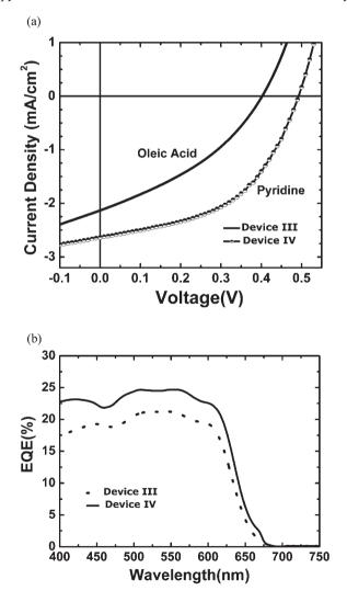
Fig. 9 (a) Photovoltaic performances of the devices before (Device III) and after (Device IV) removing the surfactant (OA) on the TiO<sub>2</sub> nanorods by pyridine treatment. Both the devices have the configuration  $ZnO/TiO_2$  nanorods/P3HT:TiO<sub>2</sub> hybrids. (b) The corresponding external quantum efficiencies (EQE) of Device IV.
