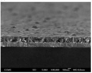
Fig. 3 Cross-sectional SEMs of (a) ZnO nanorod arrays, (b) ZnO nanorods after the infiltration of  $P3HT:TiO_2$  nanorod hybrid.
