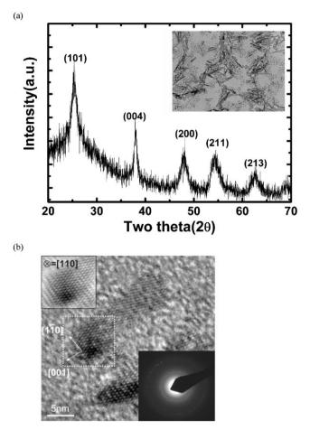
**Fig. 2** (a) X-Ray diffraction (XRD) pattern of  $TiO_2$  nanorods. The inset shows the TEM image of  $TiO_2$  nanorods. (b) High-resolution TEM (HRTEM) image of  $TiO_2$  nanorods and the corresponding selected-area diffraction pattern (inset).
