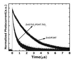
Fig. 8 Fast transient photocurrent decay for Device I (ZnO/P3HT) and Device III(ZnO/TiO<sub>2</sub> nanorods/P3HT:TiO<sub>2</sub>) respectively.
