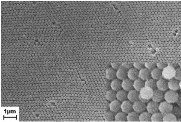
FIG. 1. SEM micrograph of silica photonic crystal infiltrated with CdSe nanoparticles. The inset shows the CdSe nanoparticles that are uniformly distributed inside the photonic crystal.
