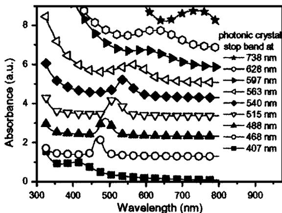
FIG. 2. Transmission spectra of nine samples of silica photonic crystals at normal incident light. The absorption peaks are changed with the diameters of silica spheres that can be varied from 407–738 nm.
