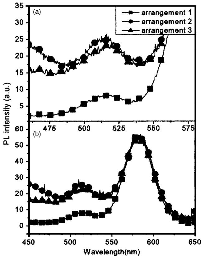
FIG. 3. Photoluminescence spectra of various arrangements of the CdSe nanoparticles with respect to the photonic crystal with stop band at 490 nm. (a) The photoluminescence intensity at 517 nm from the arrangement 2 and the arrangement 3 was greatly enhanced by 4–5 times as compared to that of arrangement 1. (b) The full spectra including the standard peak.
