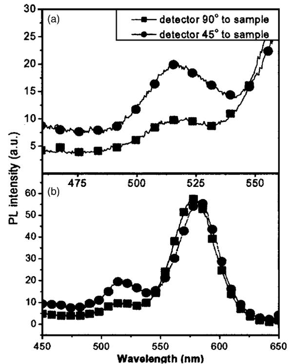
FIG. 4. Photoluminescence spectra were measured at 45° and 90° respect to the CdSe infiltrated photonic crystal with stop band at 520 nm. (a) The photoluminescence intensity of 517 nm collected at an angle of 45° is larger than that collected at an angle of 90°. (b) The full spectra including the standard peak.
