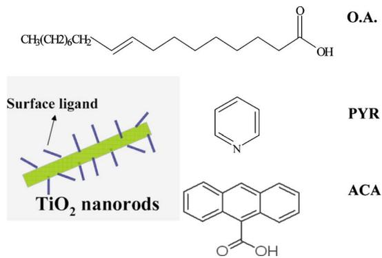
FIG. 1. (Color online) Schematic representation of three different kinds of surface ligands on the  $\text{TiO}_2$  nanorod surface.
