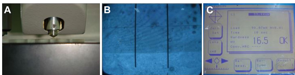
Figure 1 Microhardness test model. (A) HMV2 (hardness test machine; Hardness Ark-600, Mitutoyo Co., Kawasaki, Japan) under 98.07 mN, Vickers hardness 0.01, 10 seconds with Vickers' indenter. (B) The indentation upon epoxy nanocomposite block is calculated on the screen. (C) The result of the microhardness test is shown on the monitor and recorded. Here, the epoxy nanocomposite-duplicated bracket-like block is fixed and tested upon the bracket wing area before thermocycling.
