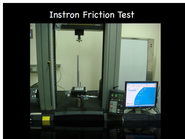
Figure 2 Friction test. Instron 5566 (Instron Co., Norwood, MA, USA) and 10-bracket model for friction test.
