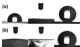
Figure 7. Change of contact angles of (a) water and (b) n -1-octadecene on the surface of the TM10Z40 nanocomposite surface after different stages of preparation; image from left to right, as cast, oxygen plasma treatment, and F-silane coating.
