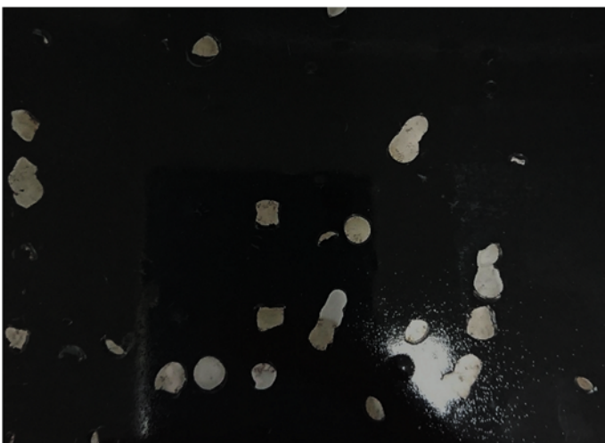
Fig. 1 Fishscaling on the surface of enameled steel.
